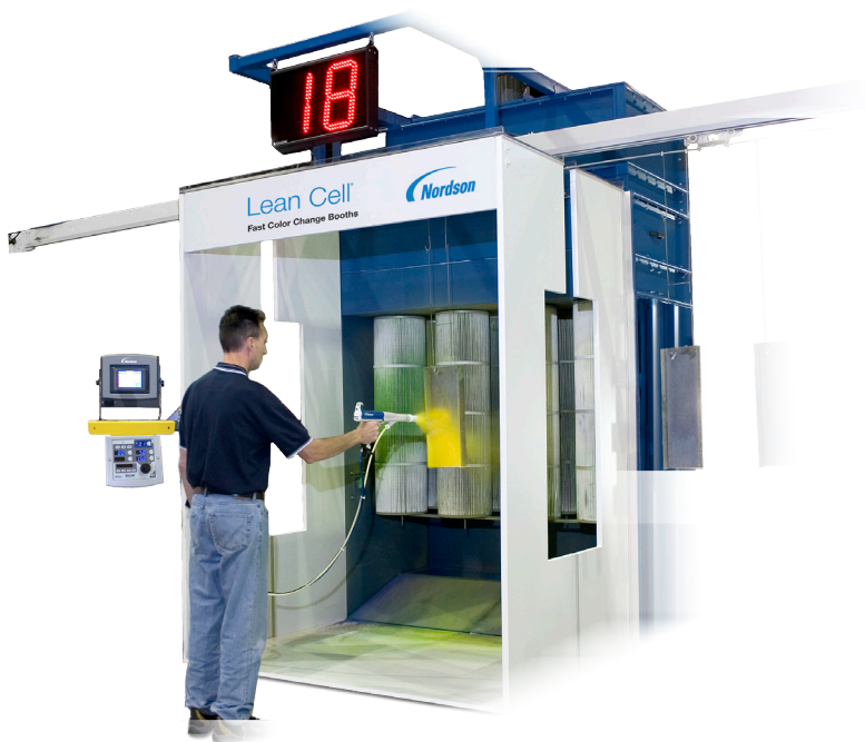
The synergy of the Nordson Lean Cell System delivers contamination-free color change in less than 20 seconds.
