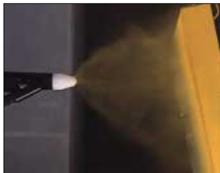
The new standard flat-spray nozzle provides better control of powder flow to deliver a more uniform pattern.
