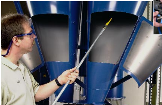
Hinged sections of the dual cyclones swing open for easy access.
