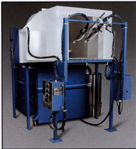
The Model 902 booth can be customized to accommodate varying automatic spray applications.
