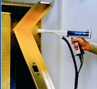
Coating Mode 2: Touch-up operations High transfer efficiency and enhanced Faraday-cage penetration
