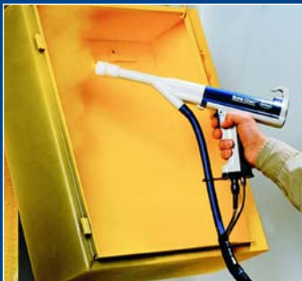
Coating Mode 3: Deep cavity areas Enhanced penetration when the gun is placed inside a cavity
