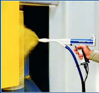
Coating Mode 1: Recoating painted parts Delays back ionization for uniform coverage and reduced orange-peel effects
